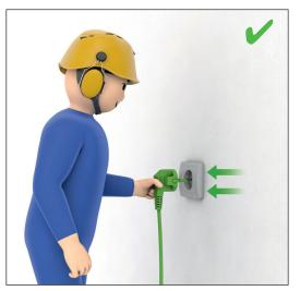
Pull the plug before working on the machine
